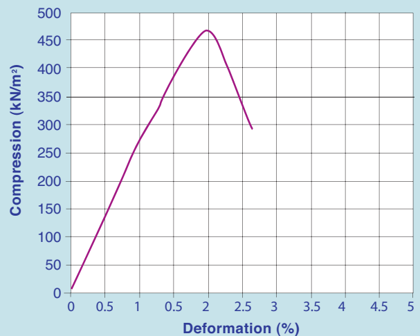
Results of Compression Test on GEOlight 400
