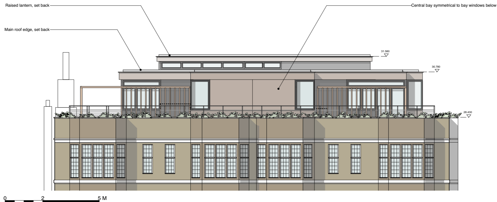
Proposed typical detailed elevation at roof level (from drawing 312.PL.016)
