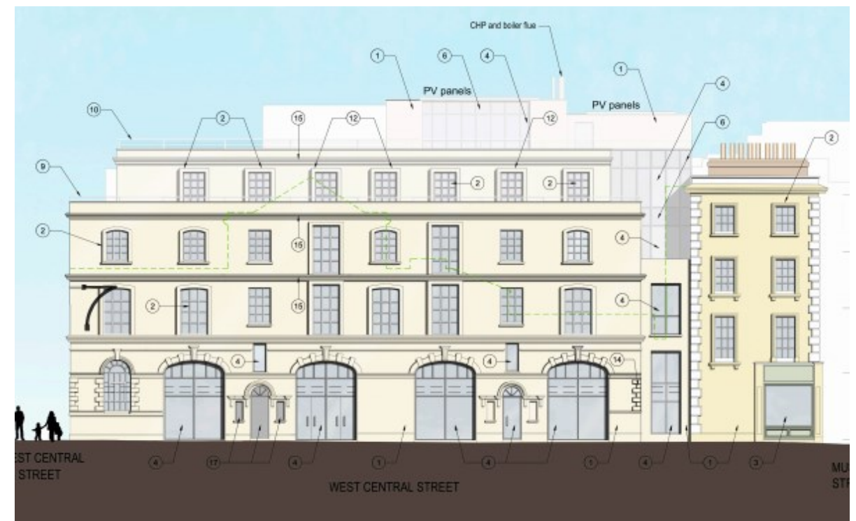
Figure 27. Detailed elevation and section drawing of no 16 West Central Street showing the proposed elevation extensions at the first, second and third floor levels.
