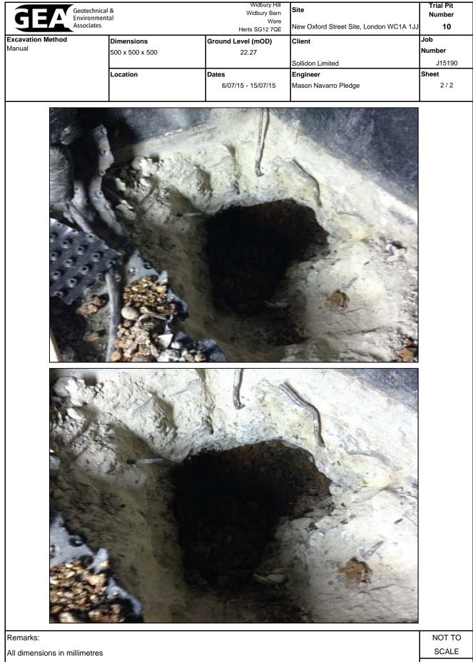
Sides of trial pit remained stable during excavation Groundwater: not encountered
