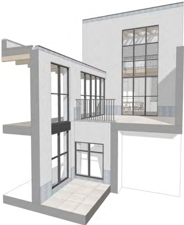
Fig. 45 - Rear Annex and Link cut away View
