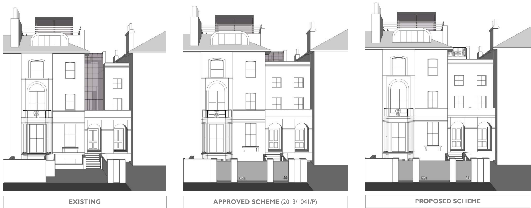
DIAGRAM 8 : Shows changes to the Front Elevation are limited to the Balustrade at Third Floor (see section 4.64 for detail)
