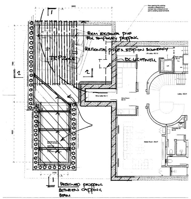
5. PROPS TO CAPPING SEAM IN PLACE, COMMENCE BLUK EXCAVATION TO RL1.
