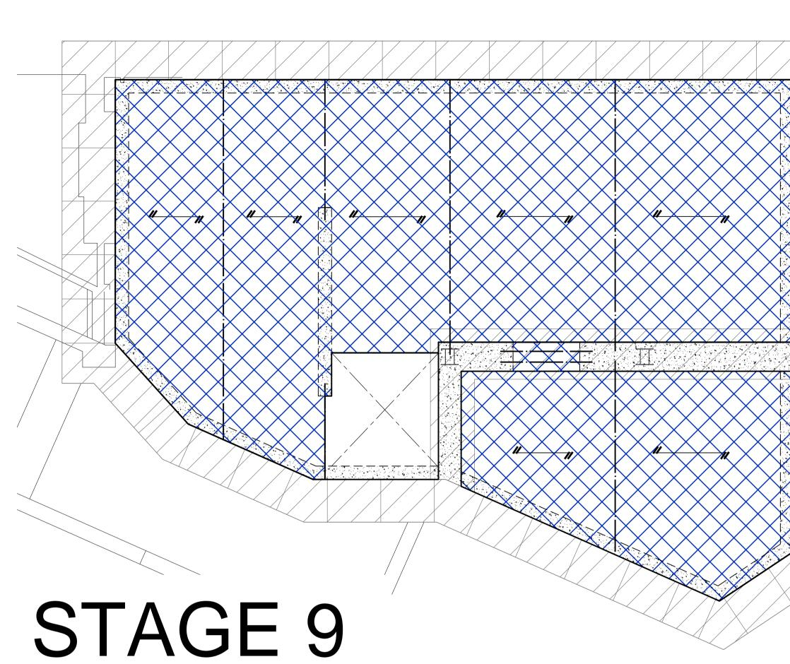
STAGE 9 ON COMPLETION OF THE GROUND FLOOR STRUCTURE THE BASEMENT INTERNAL DIAGONAL STRUTTING CAN BE REMOVED.
