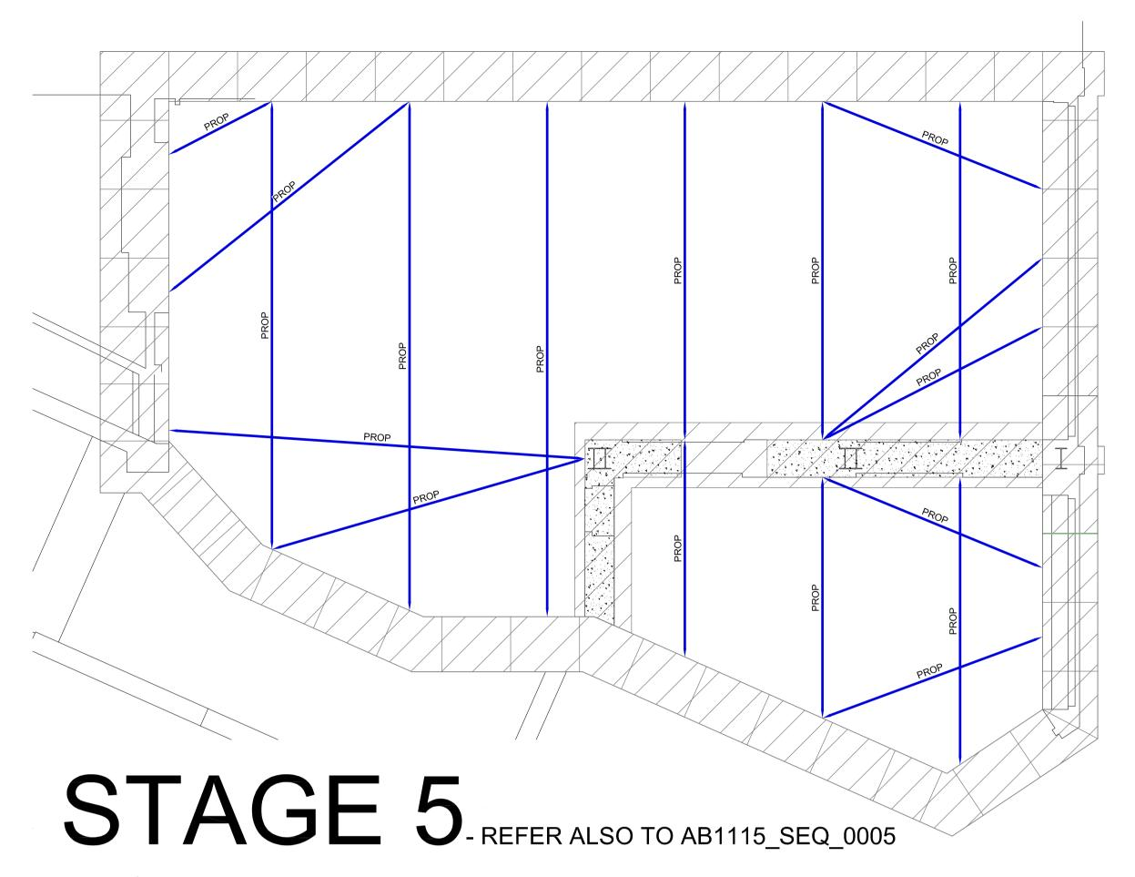
STAGE 5 TO THE PERIMETER OF THE NEW BASEMENT FOOTPRINT THE INSIDE FACES OF THE UNDERPINS WILL HAVE TEMPORARY DIAGONAL STRUTTING INSTALLED AS REQUIRED TO RESTRAIN THE TOPS OF THE UNDERPINS.
