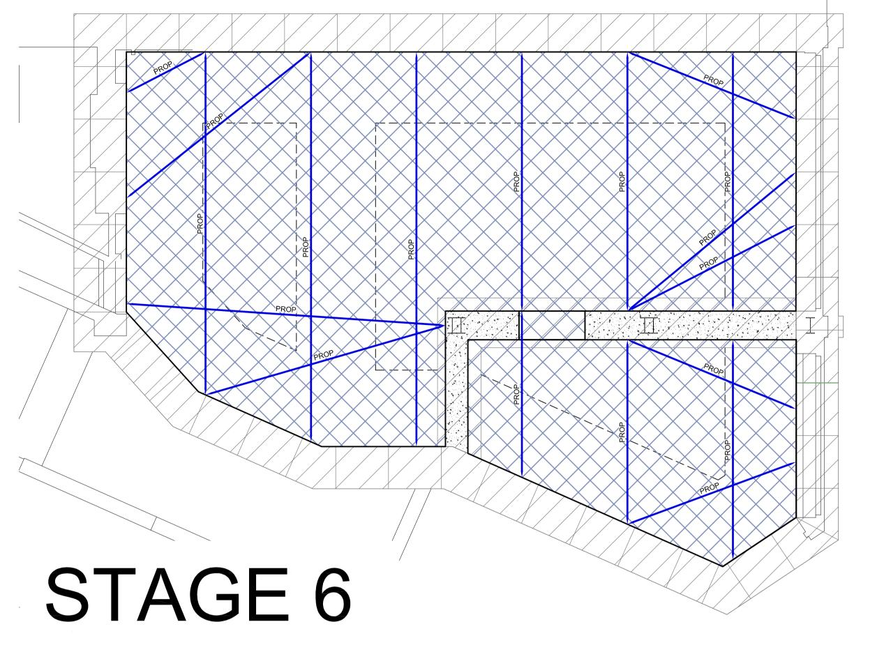
STAGE 6 CONSTRUCT NEW FOOTINGS AT BASEMENT LEVEL FOR THE NEW BASEMENT INTERNAL WALLS.
