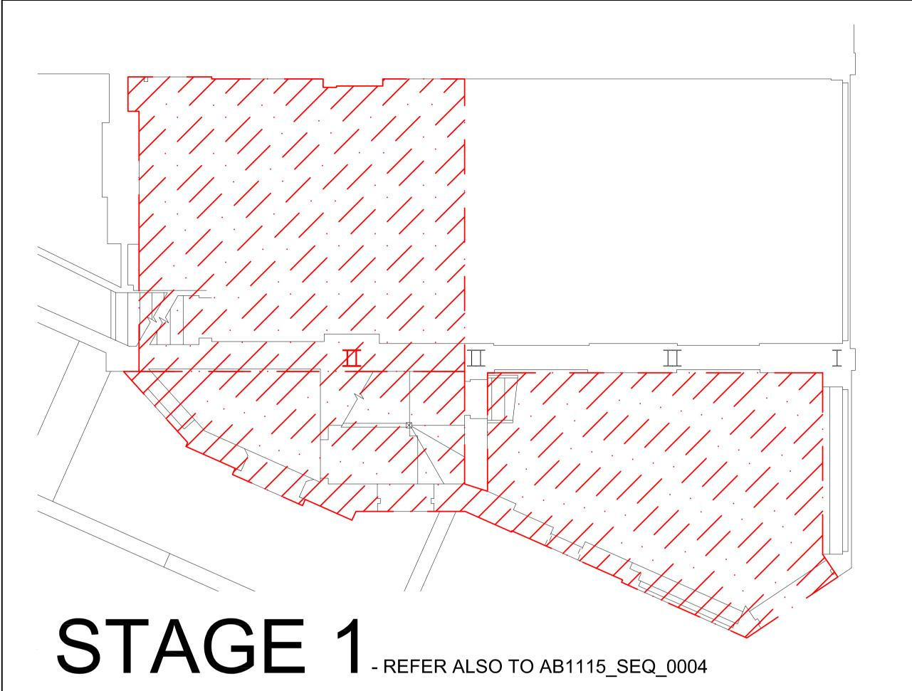
STAGE 1 DEMOLISH EXISTING SOUTH GABLE END OF THE BUILDING AND REAR SUPERSTRUCTURE OF MAIN BLOCK SOFT STRIP OF EXISTING BUILDING INCLUDING REMOVING ALL WINDOWS AND DOORS MAKE ALTERATIONS TO THE UPPER FLOORS AND ROOF
