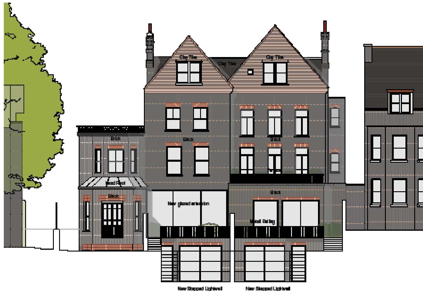
Proposed rear sectional elevation, showing proposed lightwells, glazed infill extension (centre), and the proposed amenity terrace
