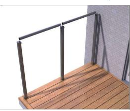
\* Glass on screens must be fixed on all 4 sides so we must run a bottom rail on the VERTICAL posts as well
