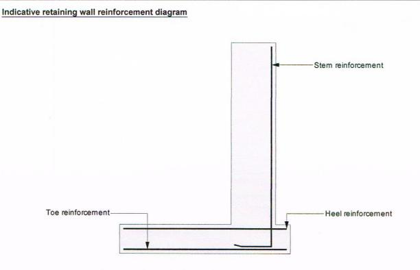
Toe bars - 16 mm dia.@ 200 mm centres - (1005 mm $^2$ /m) The design of the retaining wall heel is beyond the scope of this calculation! Stem bars - 16 mm dia.@ 200 mm centres - (1005 mm $^2$ /m)
