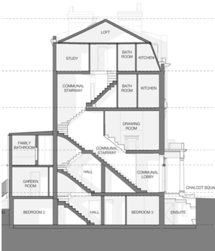
Fig 20. Existing staircase arrangement
