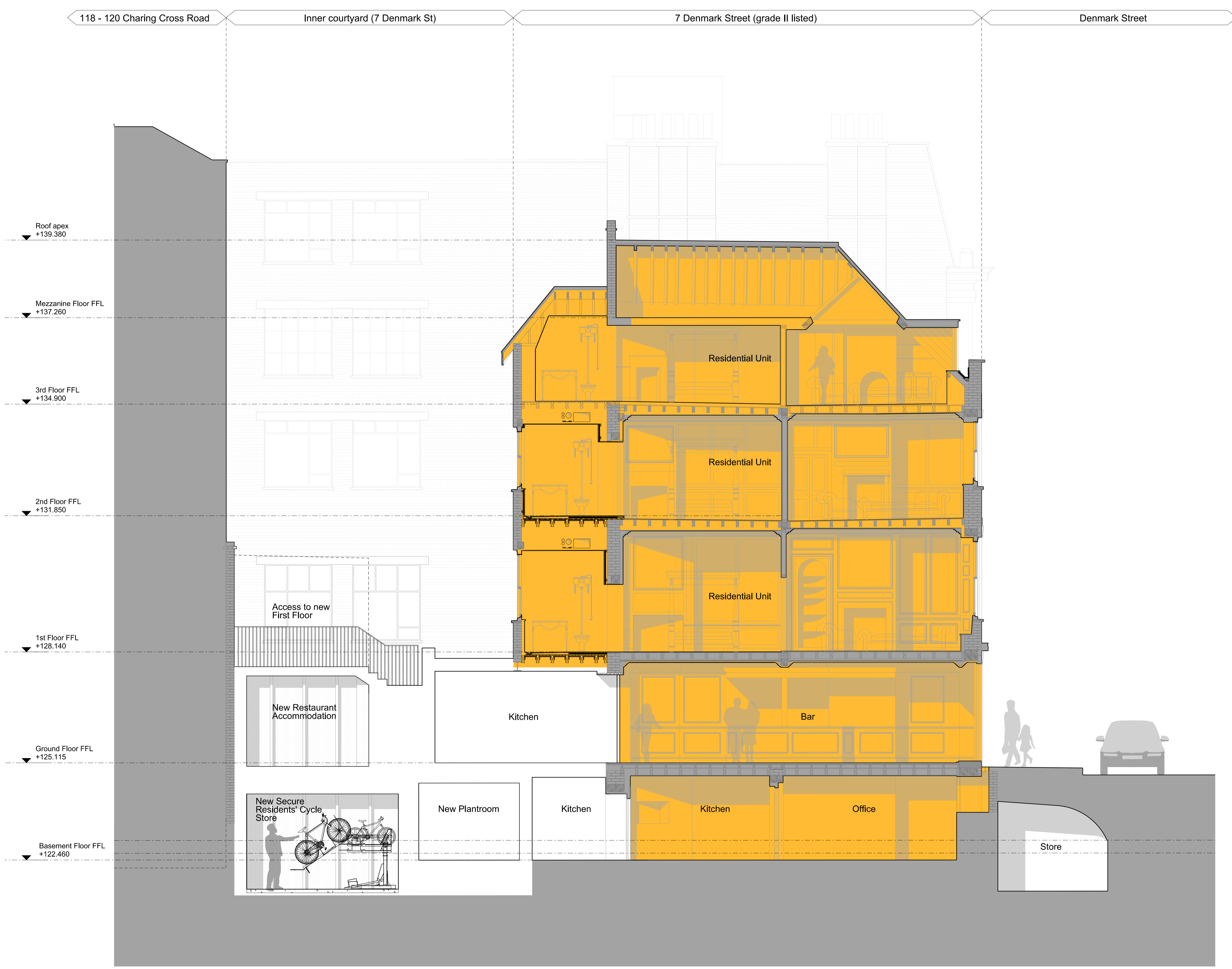
01 Proposed Section - Main House + Mews Building PL(7D)10 Looking West - at boundary wall 1:50
