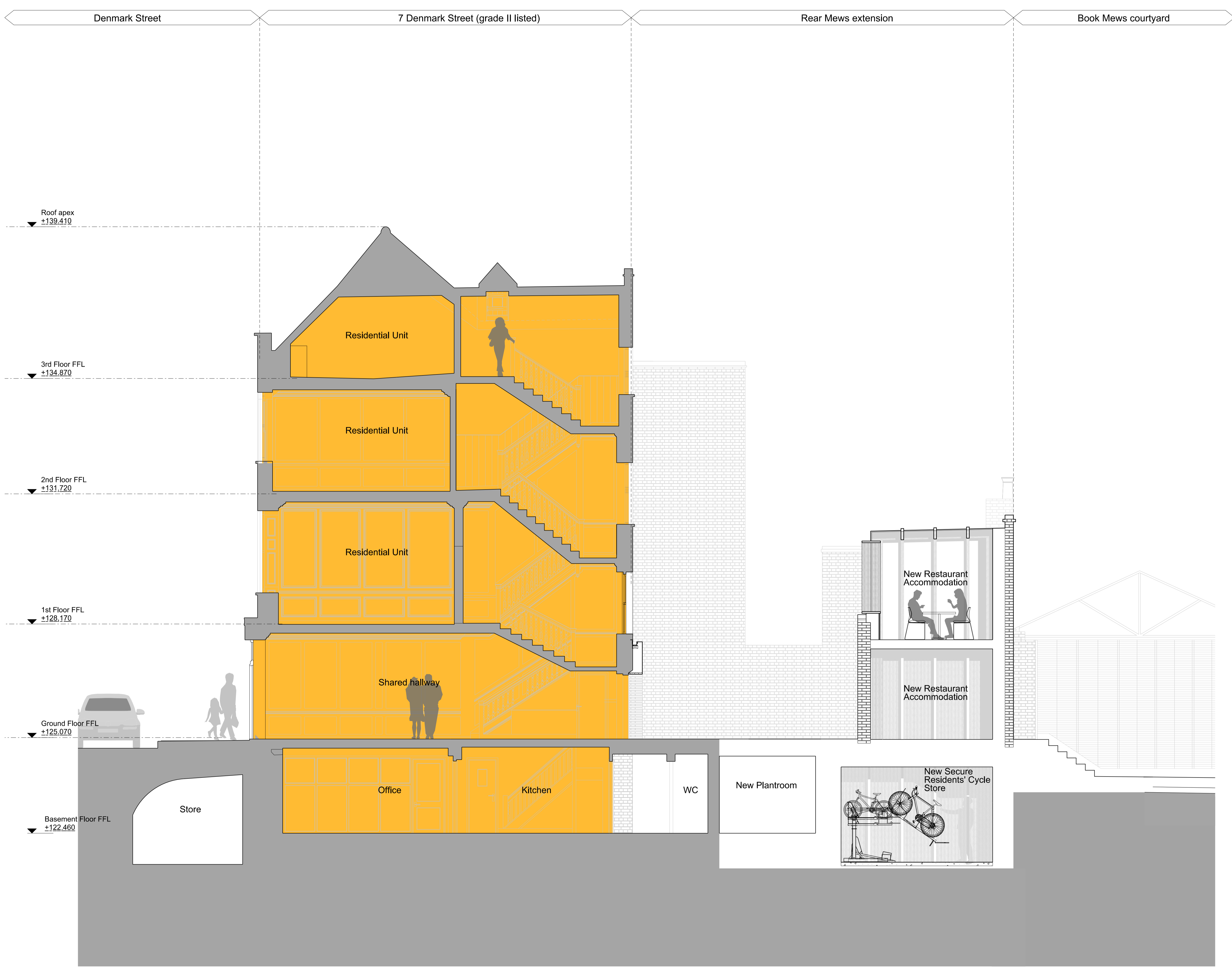
01 Proposed Section - Main House + Mews PL(7D)12 Looking East 1:50
