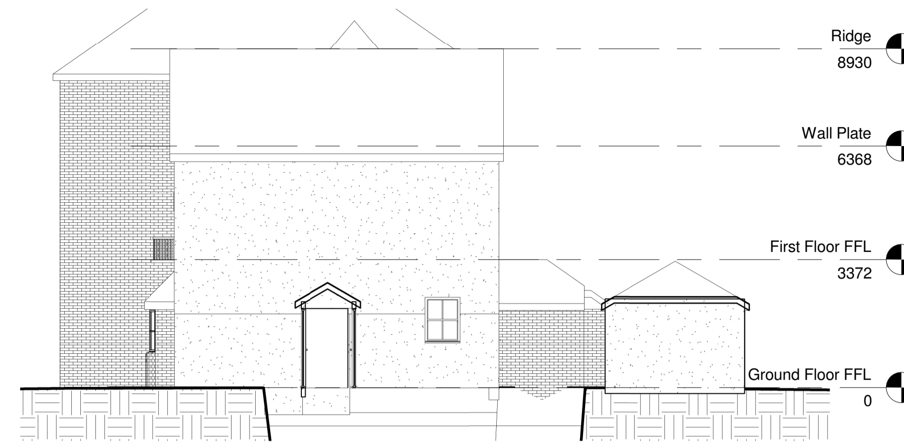
5 Existing Side Elevation 1 : 100
