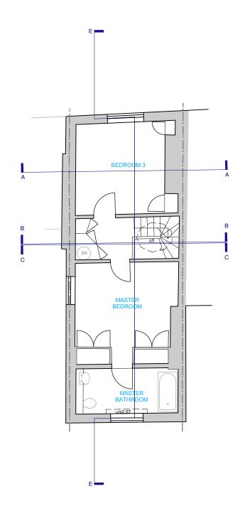
1 EXISTING FIRST FLOOR PLAN SCALE 1:100@A3
