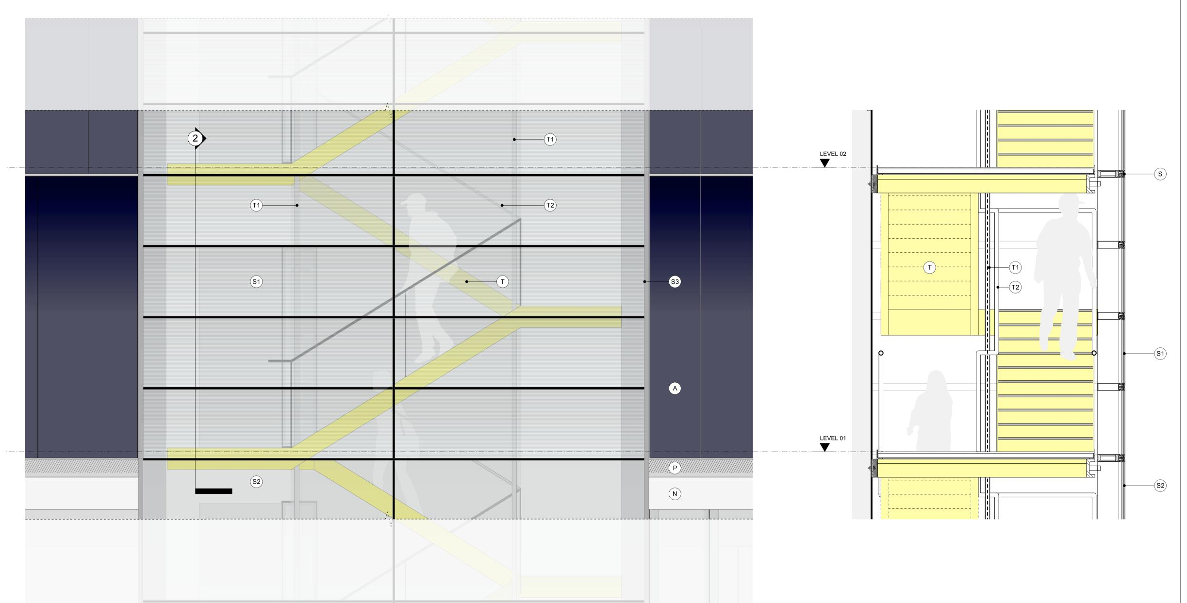
UNITISED FRAMELESS CURTAIN WALLING SYSTEM WITH CIRCA 200M DEEP GLASS RAINSCREEN FIXED TO OUTSIDE. RAL 5011 STEEL BLUE CERAMIC FRIT TO REAR (FACE 2) OF RAINSCREEN GLASS. GLASS REVEALS AROUND EDGES (TOP, SIDES AND SOFFITS) OF OVERALL RAINSCREEN ZONE TO MATCH
