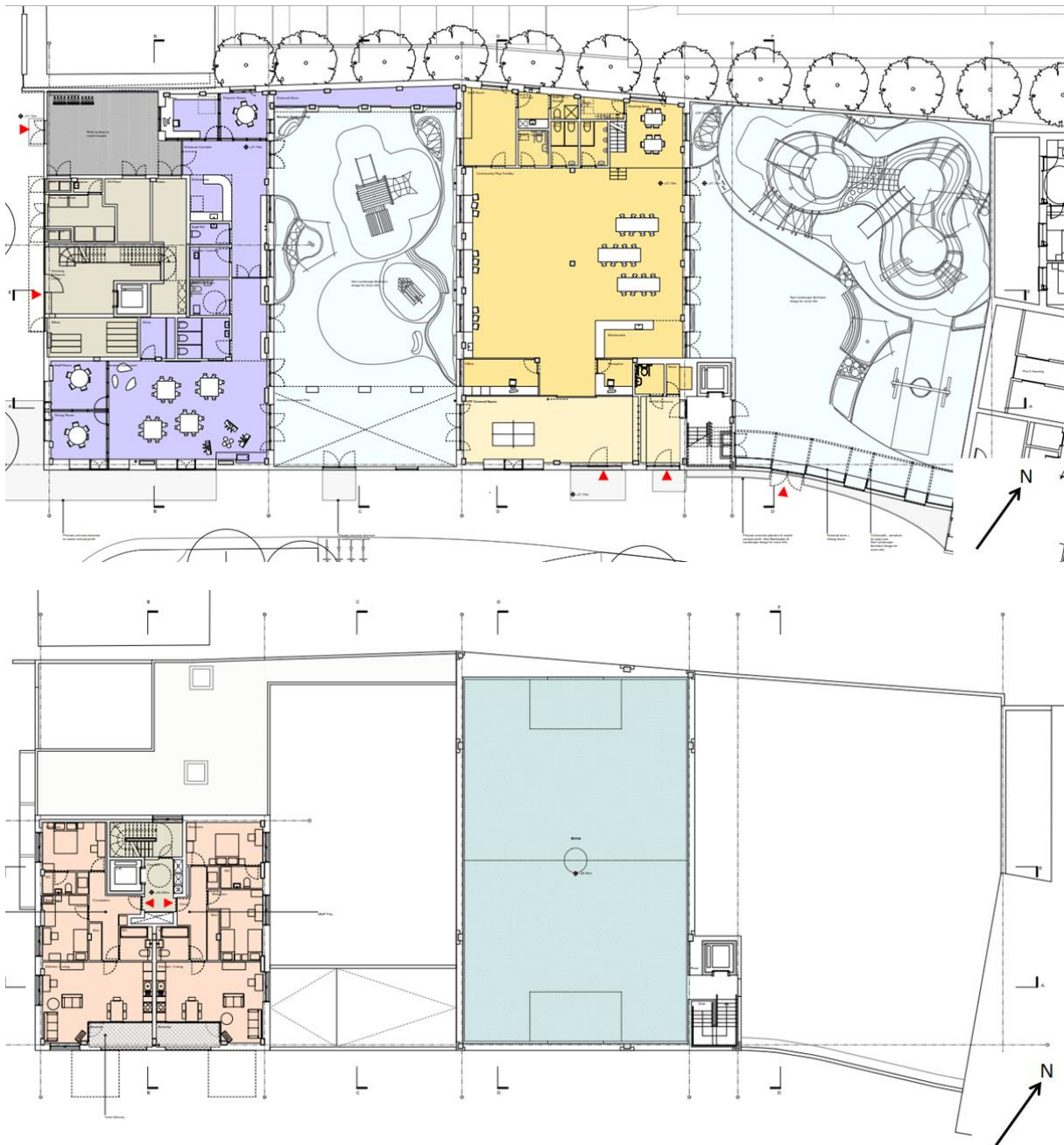
Figure 3: Footprint of proposed development. Top: ground floor. Bottom: upper floors showing indicative residential footprint (5 storeys) above Nursery, and MUGA area above Community Play Facility. Drawing as submitted for planning, 30/04/2015
