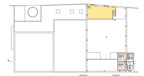
The maximum travel distance to the external stair is 25.5m in a single direction. As the MUGA is on the roof of the CPF and in external air, the travel distance is considered to be acceptable.
