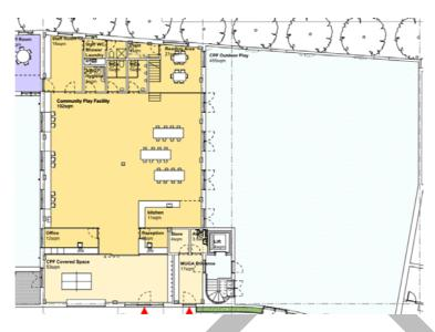
Final exits are available via the CPF covered space and via the exit doors to the external elevation onto the CPF outdoor play area. All areas are within either 18m in a single direction of escape, or 45m where more than one direction of escape is available. The gates from the outdoor play areas must be capable of being opened from the escape side without the use of a key at all material times they are required.
