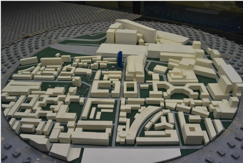
Figure B.6: Wind tunnel set-up, viewed from downstream
