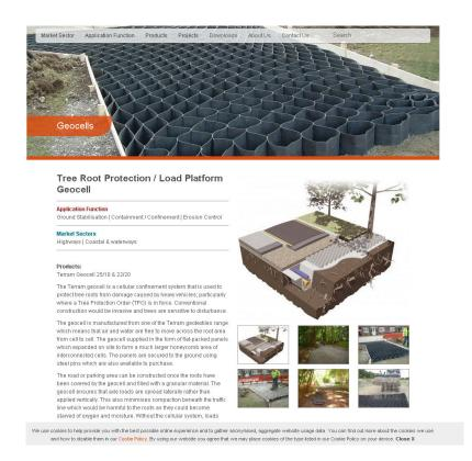
An example of suitable ground protection within trees RPA would be the TERRAM Tree root protection geocell.
