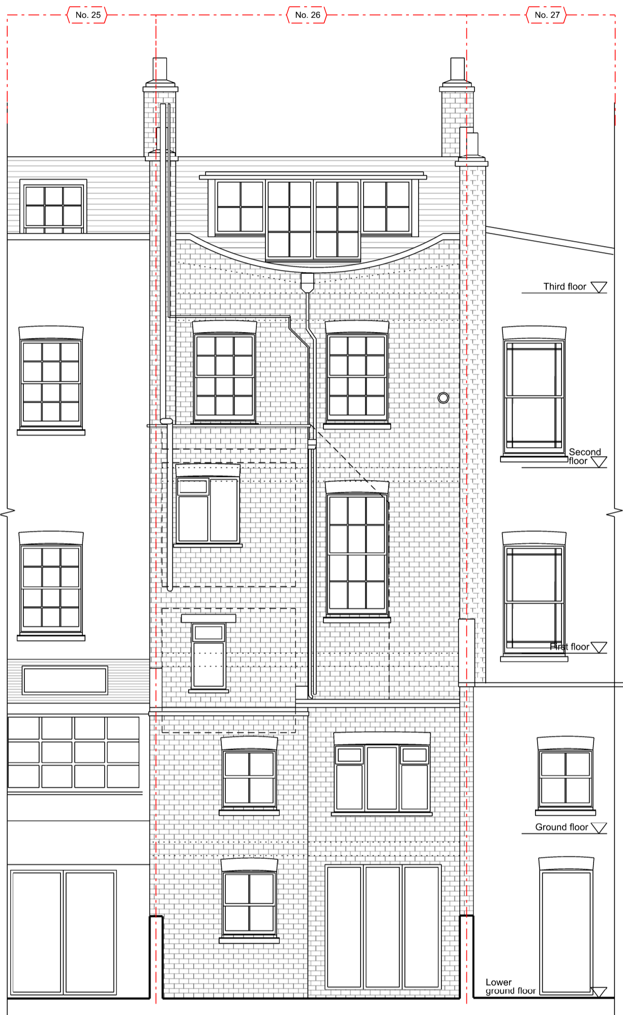
EXISTING REAR ELEVATION
