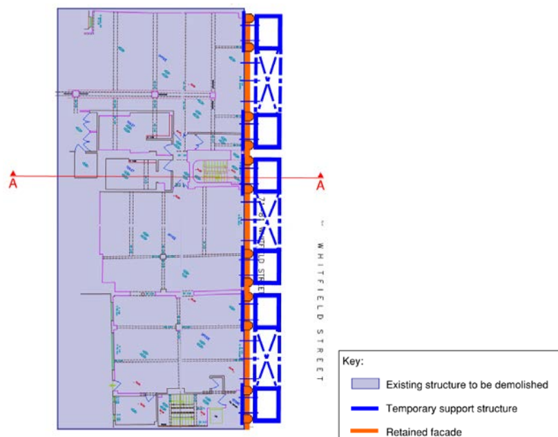
Figure 3 - Envisaged 71-81 Whitfield Street façade support arrangement
