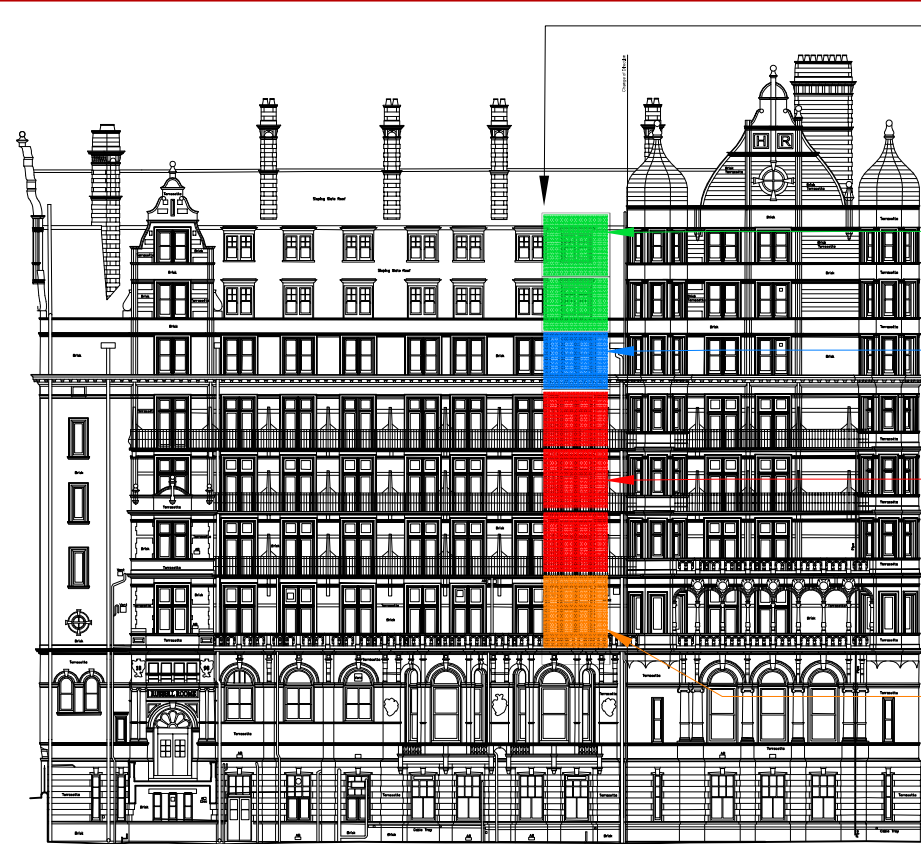
LOCATION OF HOIST - BERNARD STREET ELEVATION, NTS
