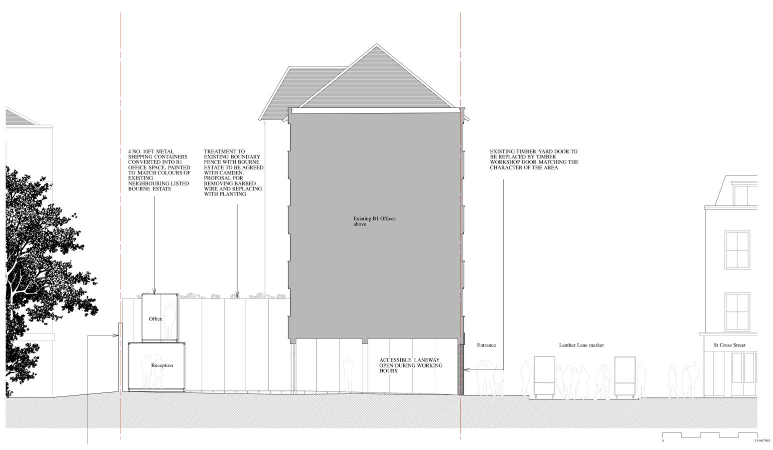
EXISTING NEIGHBOURING WALL TO REMOVE BARBED WIRE PROTECTION AND TO BE BUILT UP IN BRICKWORK TO MATCH EXISTING
