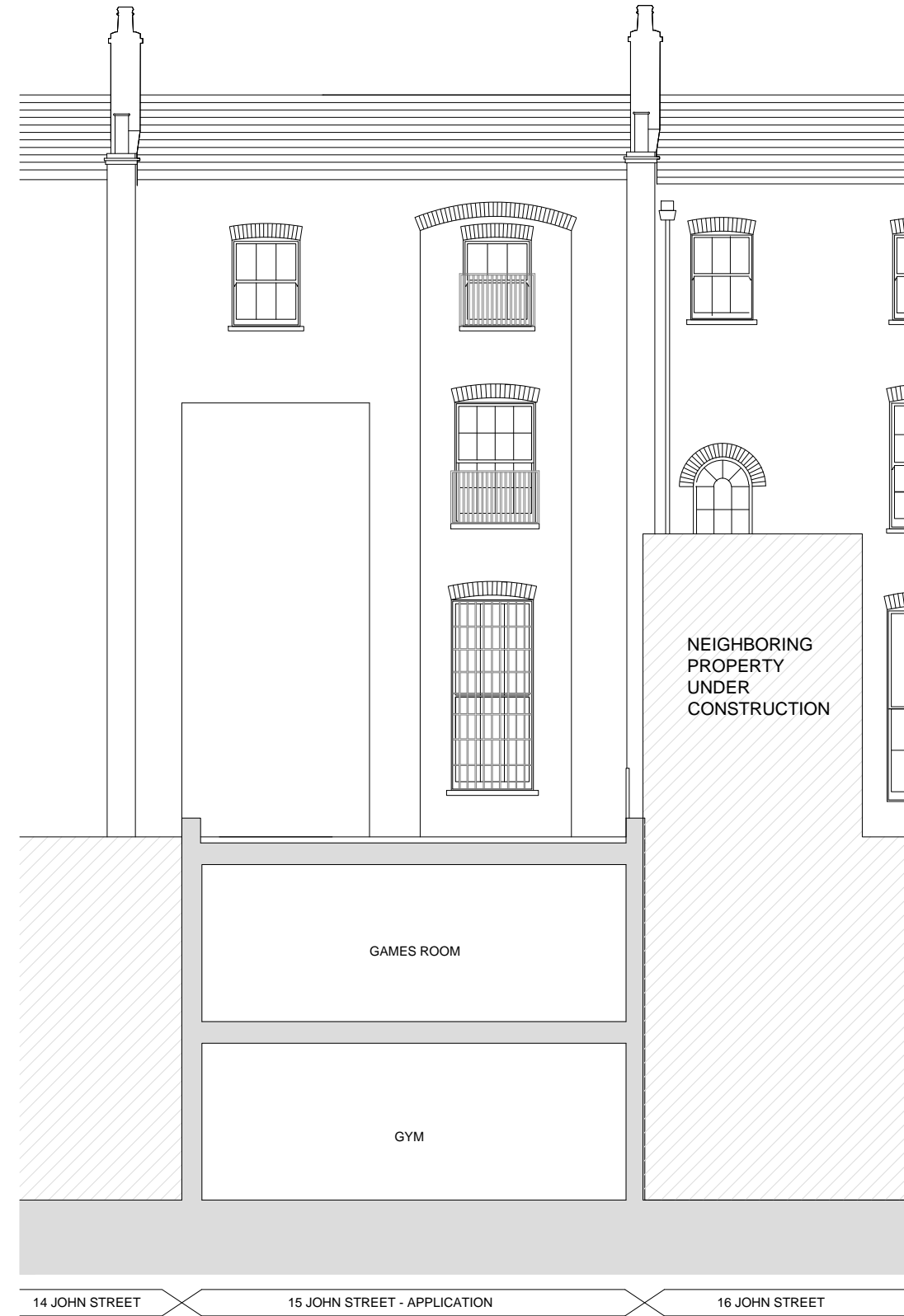
EXISTING REAR ELEVATION
