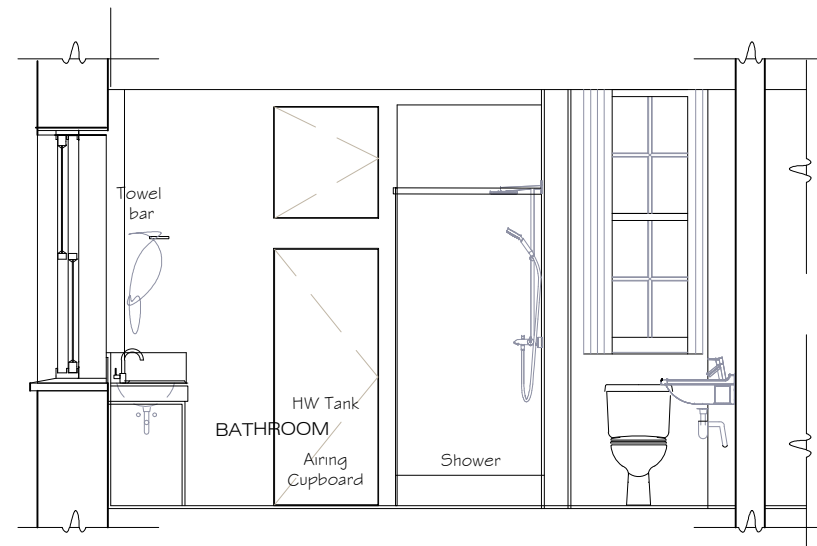
EXISTING ELEVATIONS FIRST FLOOR DETAIL 01
