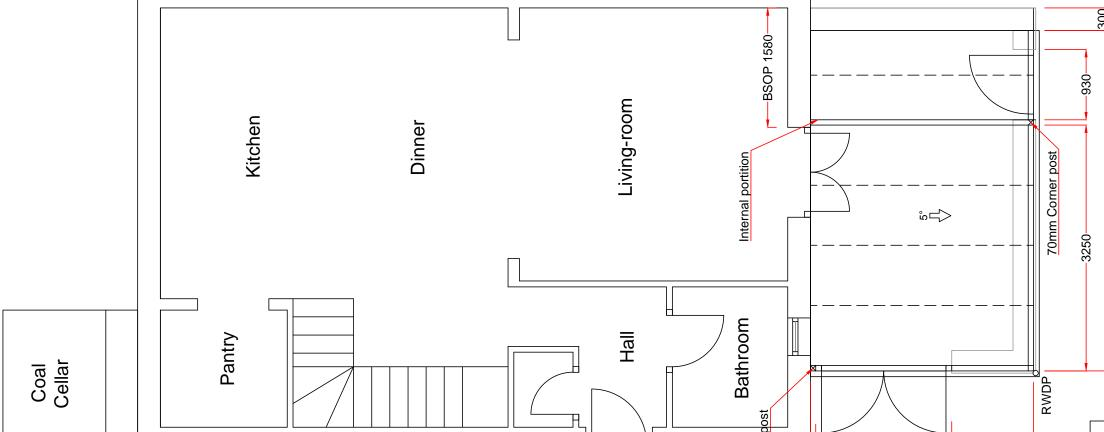
Any drawings or plans depicted make no allowance for the provision of any tie bars within the roof of the proposed conservatory. This can only be determined once the roof is put into manufacture.
