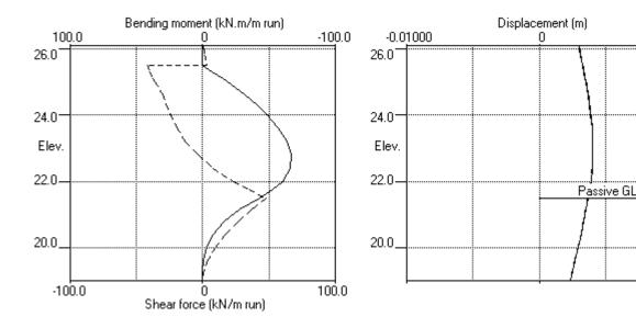
Stage No.6 Excav. to elev. 21.50 on PASSIVE side
