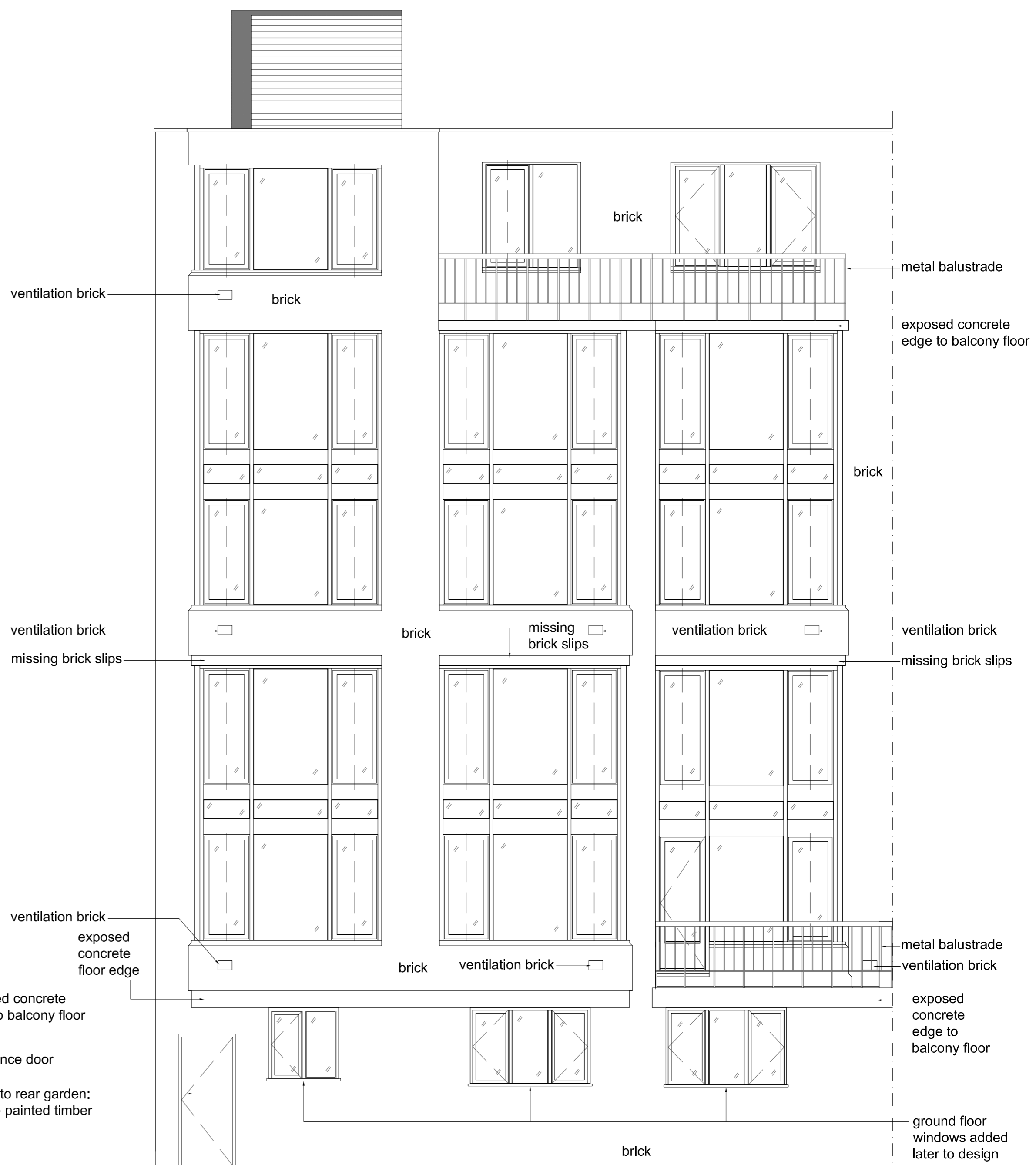
REAR ELEVATION FACING SOUTH-WEST
