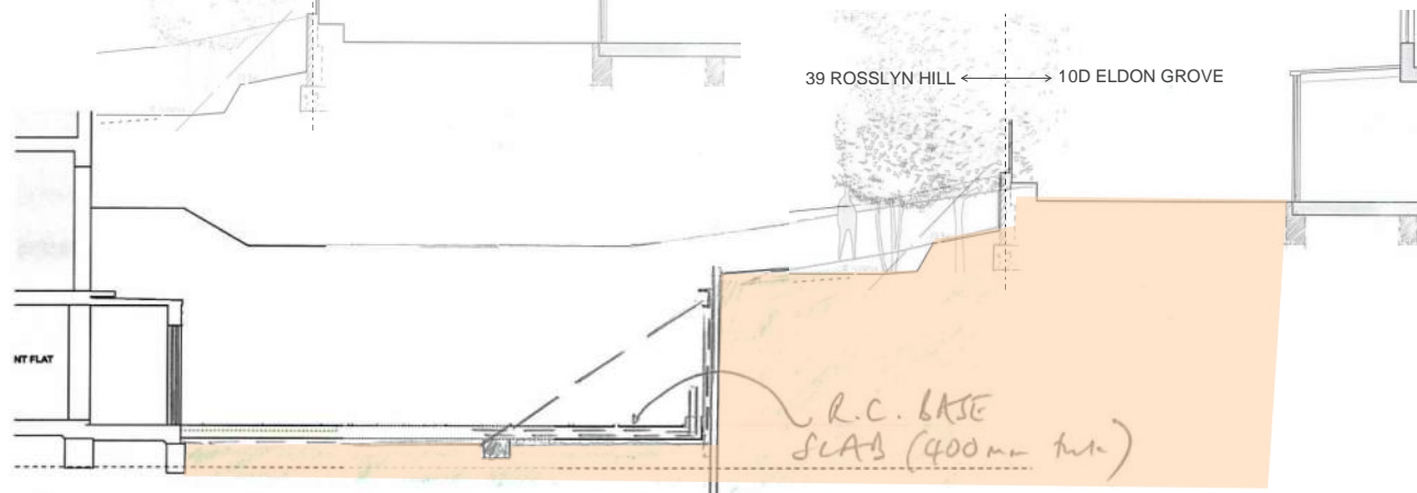
4. BASE SLAB CAST INCLUDING STARTER BARS TO RETAINING WALL
