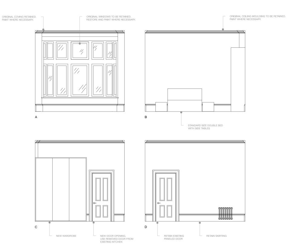
This drawing is the copyright of Red Squirrel AK Ltd. T/A Camouflage. Figured dimensions to be taken in preference to those scaled. All dimensions to be checked on site before any work proceeds. The contractor is to provide full size setting out drawings based on the information contained in this drawing for the designer approval prior to commencing manufacture. This drawing is issued on the
