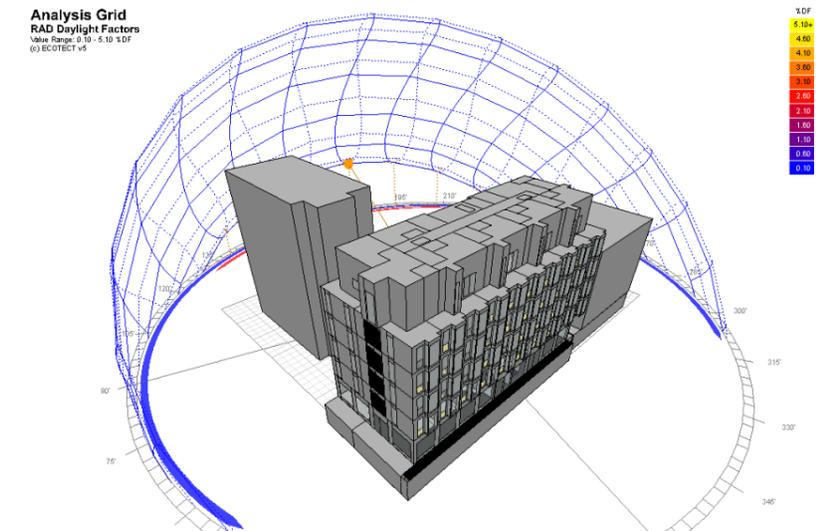
A daylighting model of the proposed development was created to maximise the use of daylight, the design intent is to compliment the current daylighting provision with lighting controls that provide artificial lighting only when needed. Similar lighting control strategies are employed on the ground floor spaces and in the living room of each apartment.
