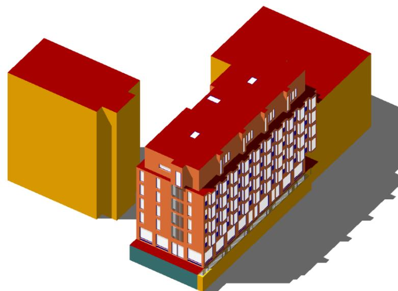
Using this model, TAS will generate a Notional Building with standardised building performance characteristics from the national calculation methodology (NCM) that will then be used as a base case upon which the proposed building will be compared. The basis of comparison will be the resulting annual emissions rate used in the energy hierarchy discussed earlier in earlier sections of this report.
