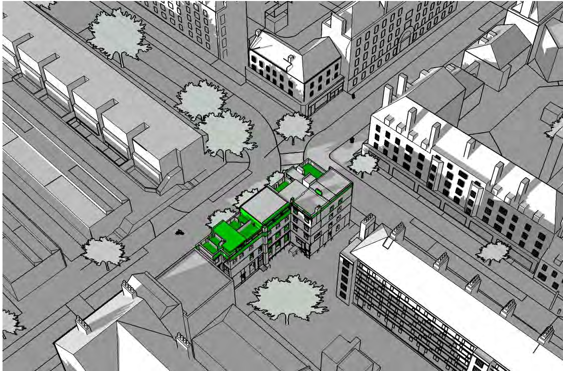
Shadow Diagram - 17.00 hours as existing on the Equinox
