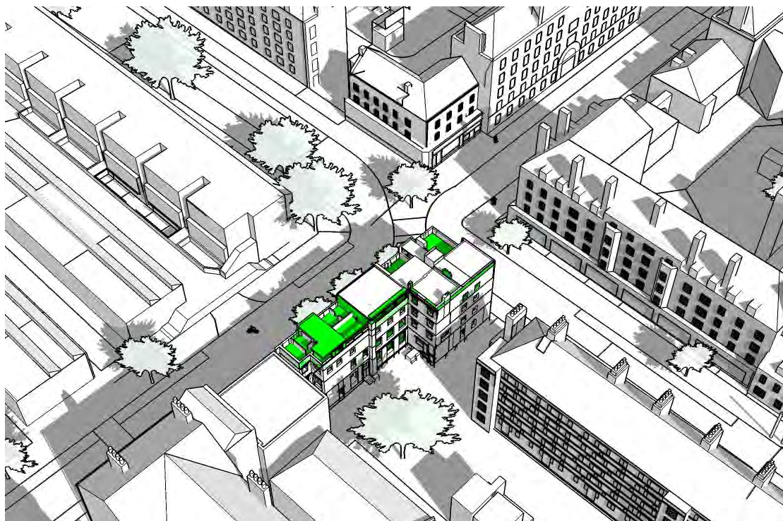
Shadow Diagram - 11.00 hours as existing on the Equinox
