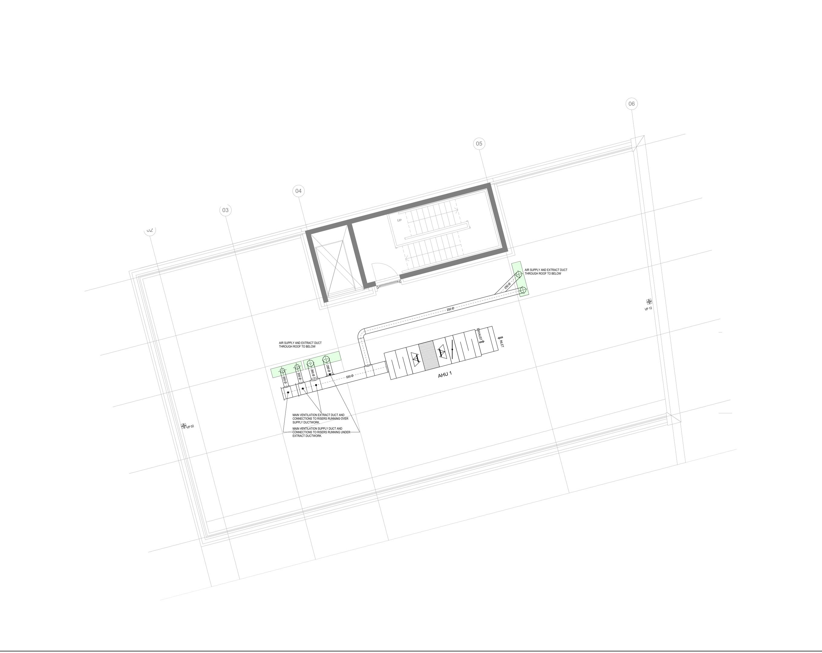
AHU 1: SWEGON GOLD RX - 11 SUPPLY/EXTRACT AIR FLOW 0.523 m3/s WEIGHT: 1026 Kg DIMENSIONS: H x W x D: 1495 x 4824 x 1199 (mm) 1. AHU TO BE ON 150mm HIGH CONTINUOUS CONCRETE BASE. 2. DUCT SUPPORTING AND RISER RAIN PROTECTION IN ACCORDANCE WITH MANUFACTURER'S INSTRUCTIONS.
