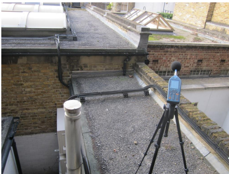
Figure 5 –Measurement Position P1 used for determining background noise levels ( L_{A90} ) in the absence of existing condensers
