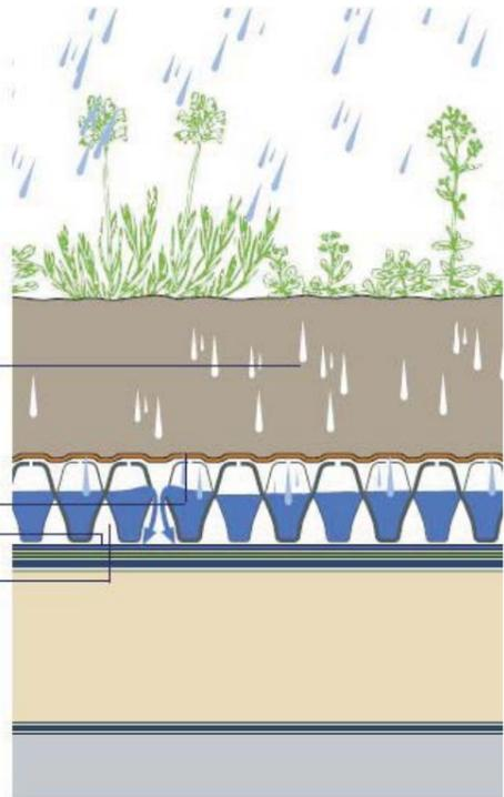
Fig 9: How a green roof releases moisture
