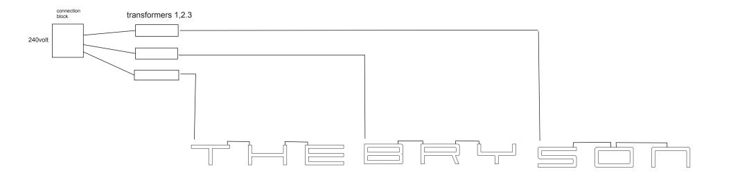
Connect all 3 transformers positive and negative 240 cables to your 240volt powder supply. using a connection box.
