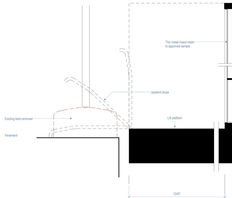
2 Platform Lift Detail - Threshold
