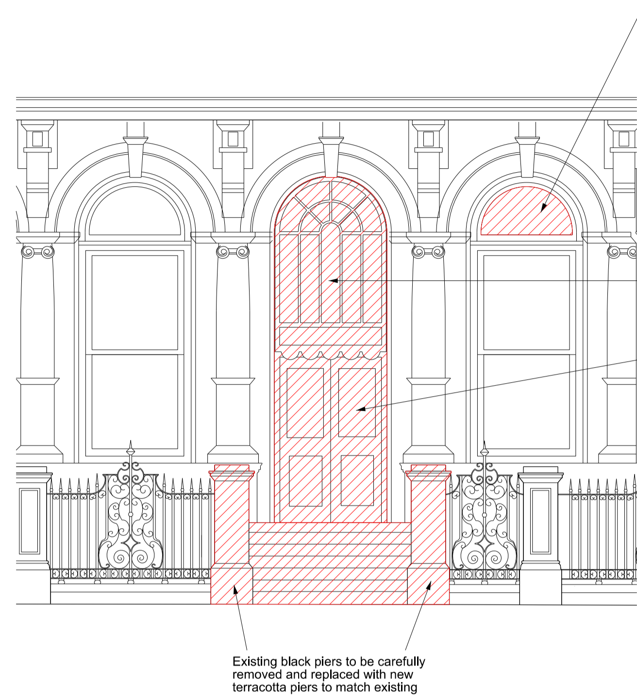
EXISTING FRONT ELEVATION
