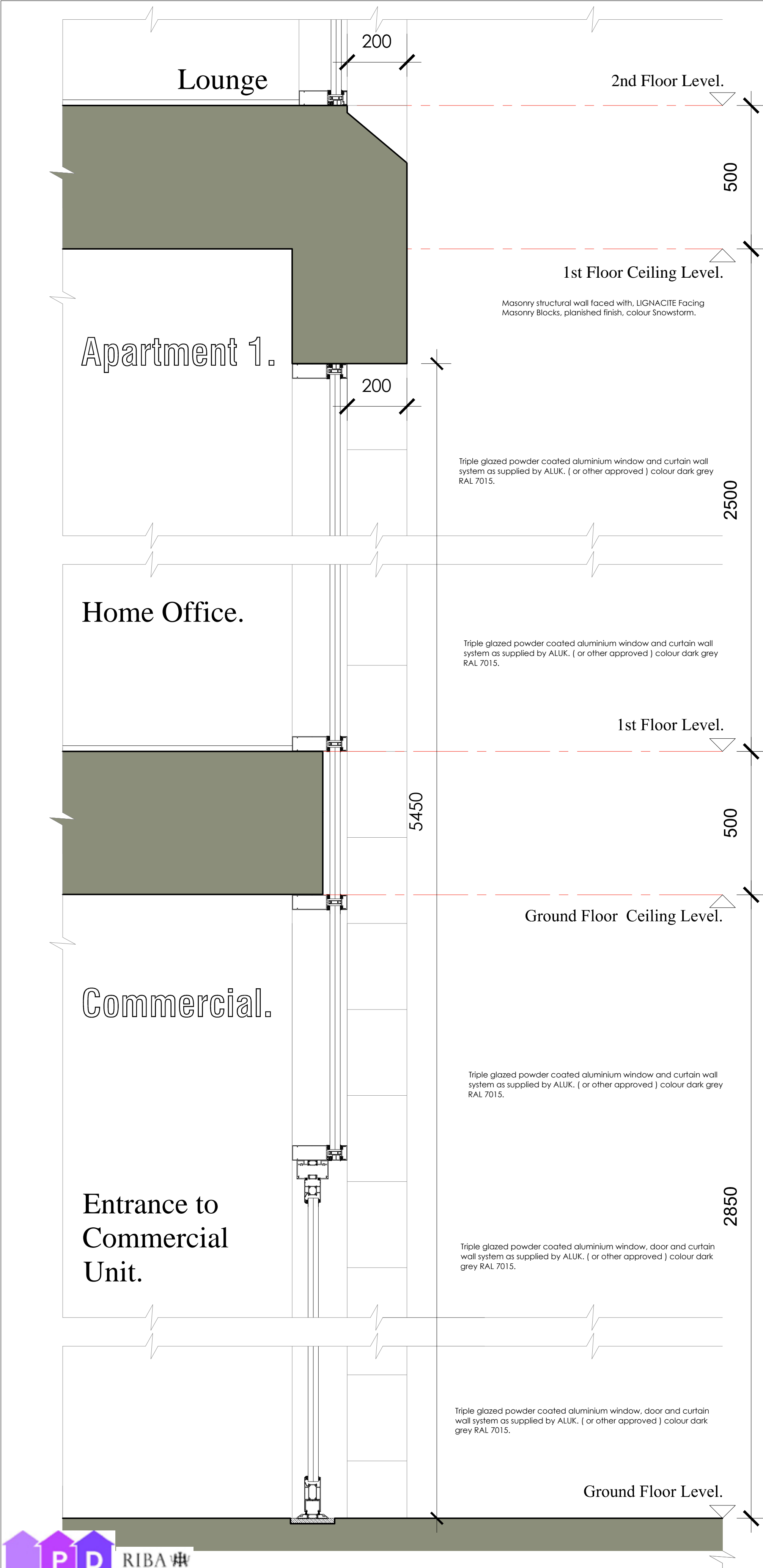
Window Door Section 4.-4. to Warren Street. scale : 1 : 10.
