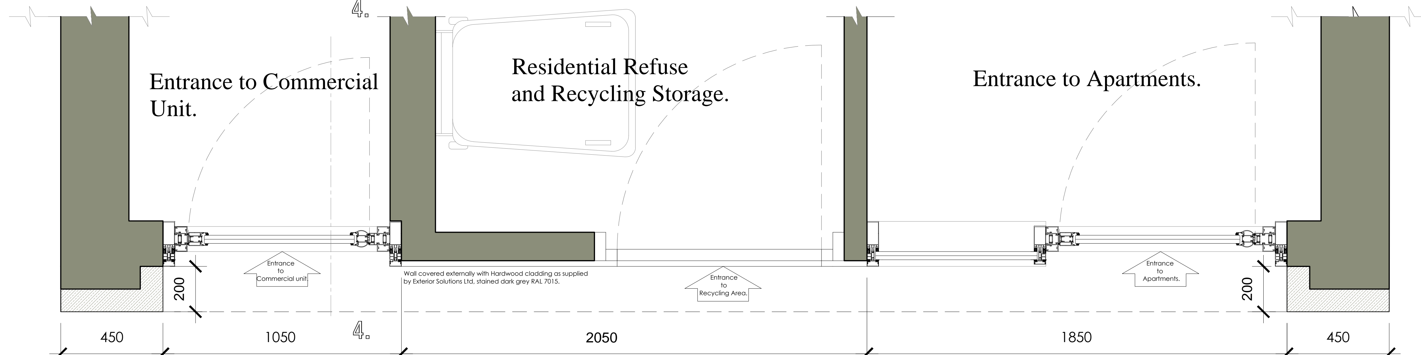
Typical Window PLAN Section: Ground Floor Level to Warren street.
