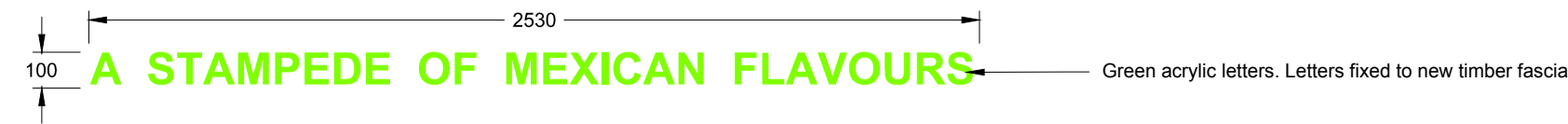
EXISTING STRAPLINE SIGN SCALE 1:20
