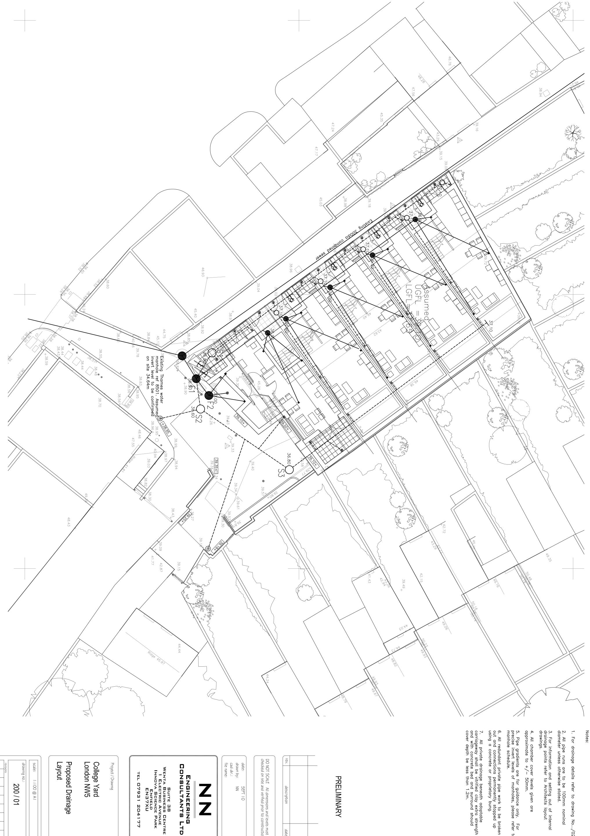
2. All pipe runs are to be 100mm nominal diameter unless otherwise stated. 1. For drainage details refer to drawing No.../02
