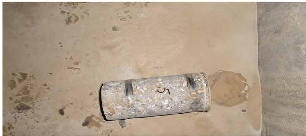
Core 5 to vault V1 (reinforced wall with sand fill behind) N.B. This vault also has had a trench cut through it for the passage of a water main.
