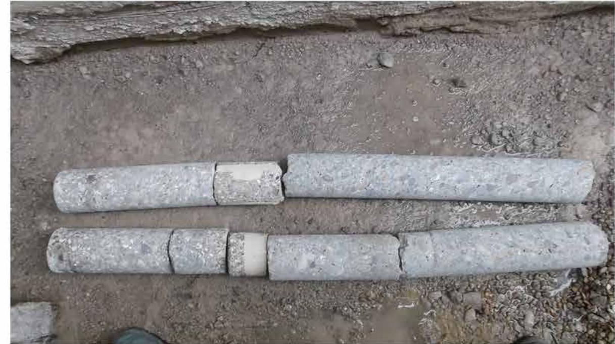
Cores 7 and 8 to vault V4: (vault totally filled with mass concrete)
