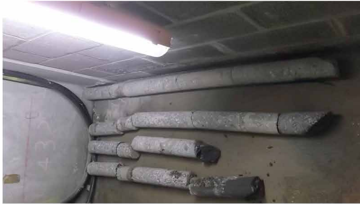
Cores 1 - 4 to vaults V2 and V3: (vaults totally filled with mass concrete)
