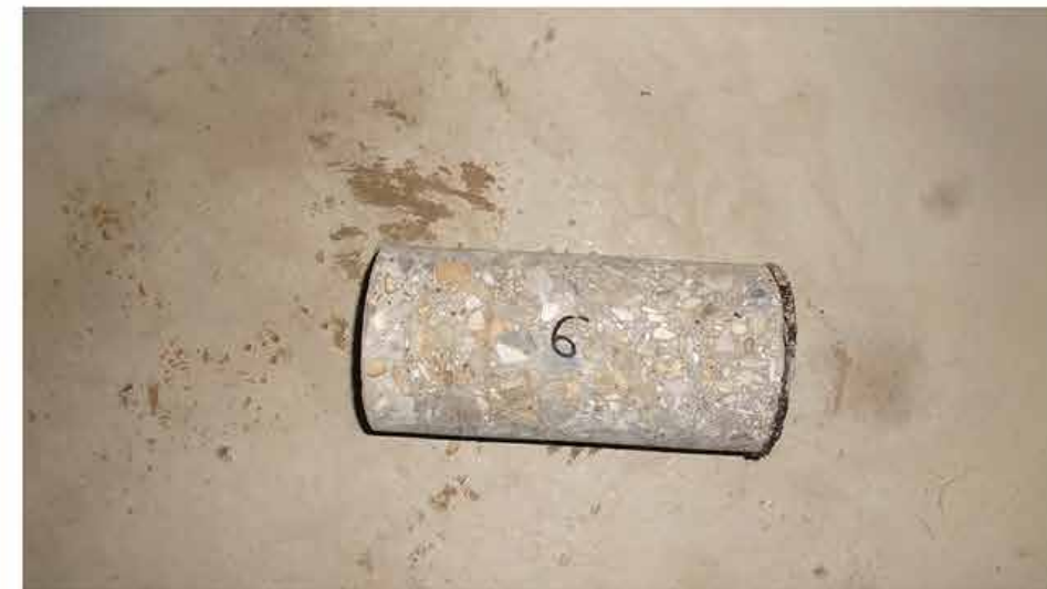
Core 6 to vault V1 (reinforced wall with sand fill behind) N.B. This vault also has had a trench cut through it for the passage of a water main.
