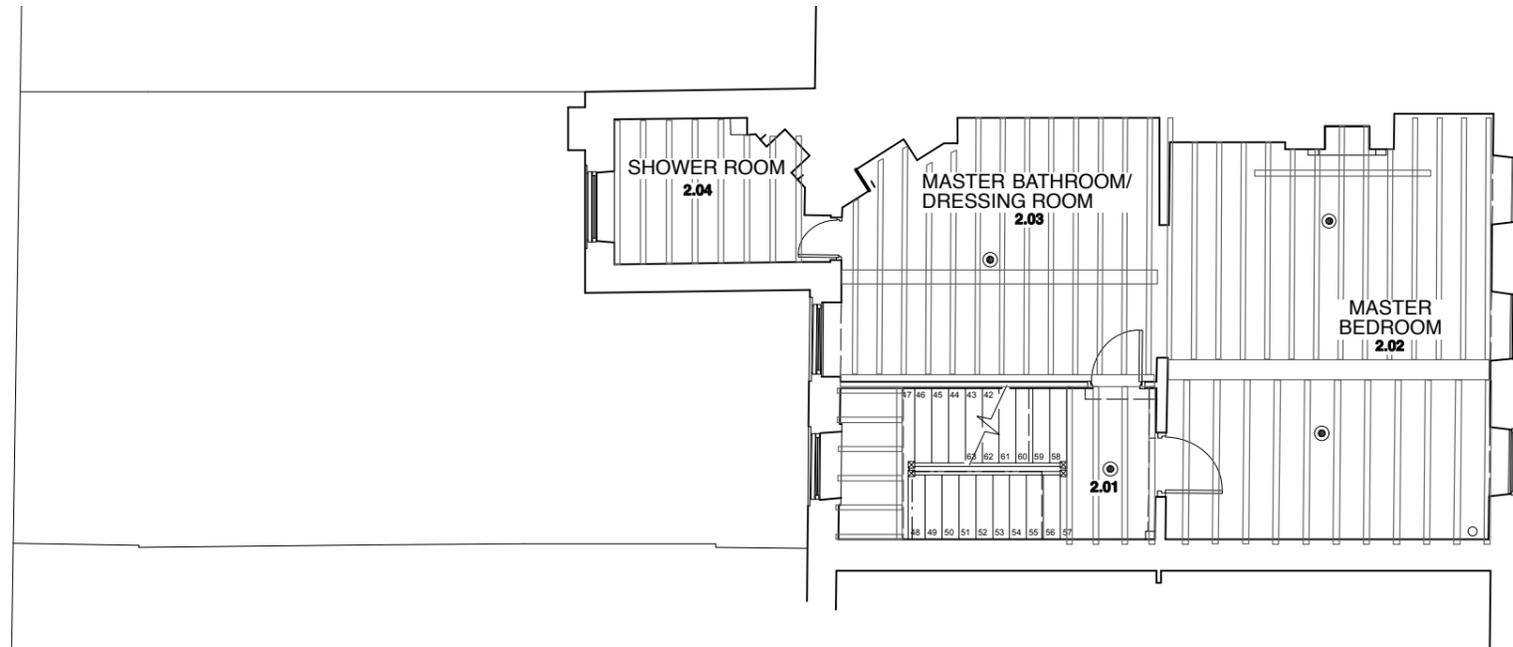
PROPOSED SECOND FLOOR PLAN SHOWING FLOOR SPRINKLER LAYOUT ON THIRD FLOOR JOISTS
