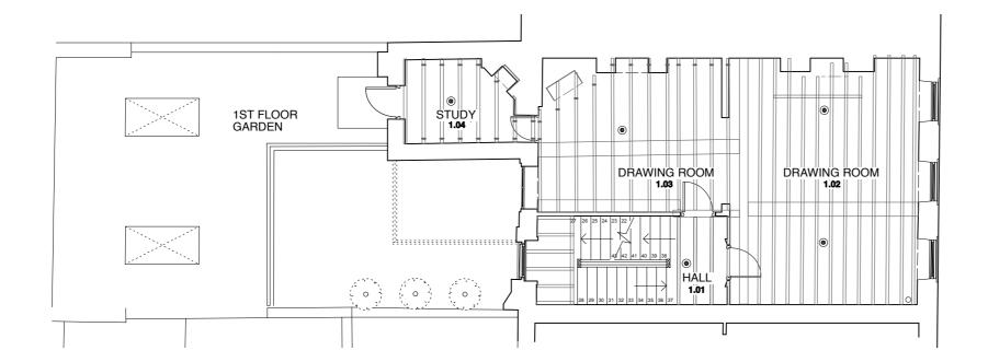
PROPOSED FIRST FLOOR PLAN SHOWING SPRINKLER LAYOUT ON SECOND FLOOR JOISTS
