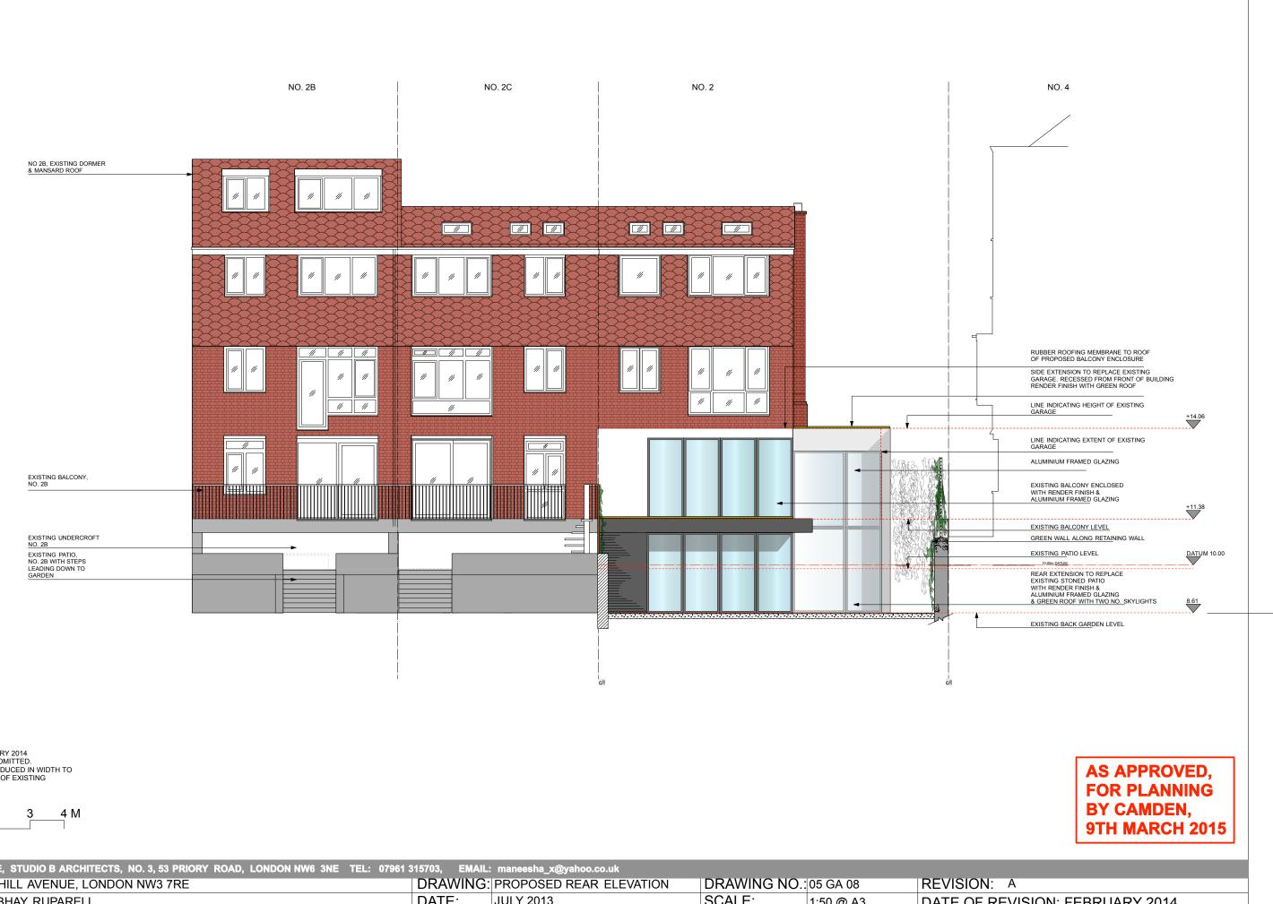
NOTES REVISION A: FEBRUARY 2014 ROOF CONVERSION OMITTED. REAR EXTENSION REDUCED IN WIDTH TO LINE UP WITH WIDTH OF EXISTING BUILDING
