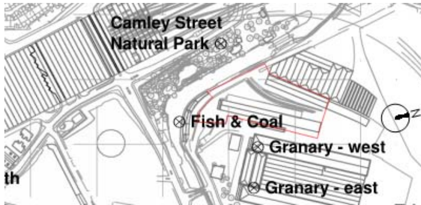
Figure 2: Baseline Noise Monitoring Locations (site outlined in red)
