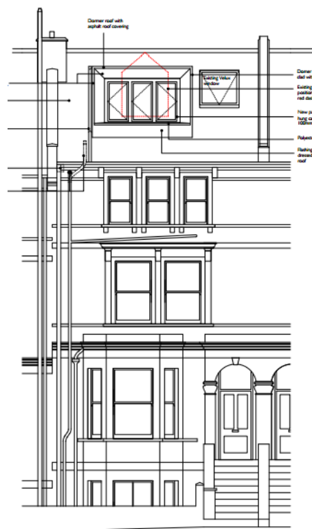
Above: front dormer enlargement approved in 2014 at 41 Montpellier Grove. The acceptance of thick edges and lack of vertical alignment shows how varied the terrace is in terms of front dormer designs.
